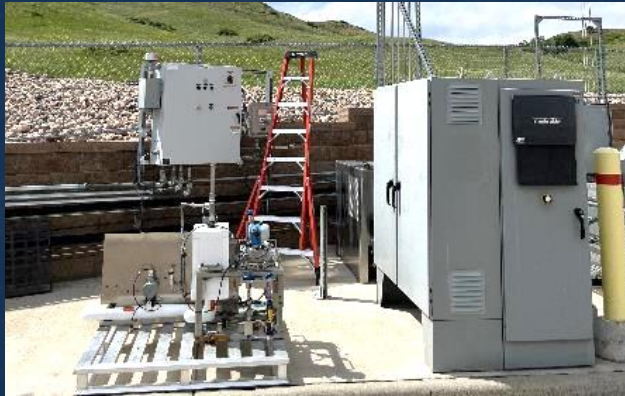
Verne's 1 tpd cryo-cooler during testing at NREL
